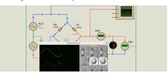
At introductory levels, simple animations for voltage levels on pins and current flow can be turned on to help students visualise what is happening. As students advance they can use basic meters to take measurements and then be introduced to instrumentation such as an oscilloscope or logic analyser for analysis. Advanced students can then work with more complex circuitry and use graphs to perform a host of more detailed analyses such as frequency, fourier or distortion.
