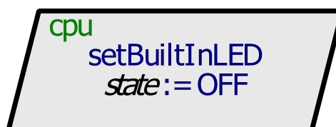
Figure 2-22: setBuiltInLED routine with "state" set to "OFF"
