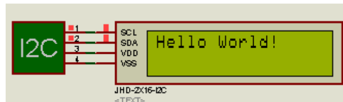
Figure 4-6: "Hello World!" displayed on LCD
