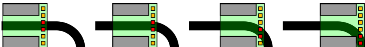
Figure 11-9: Changing line position as robot drives forwards
