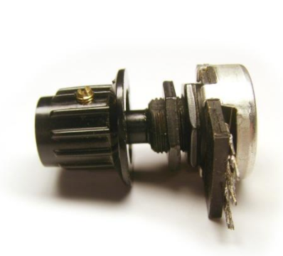
Figure 7-4: Potentiometer with knob
