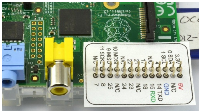
Engraved casing or simple template to identify lines on the header block.
